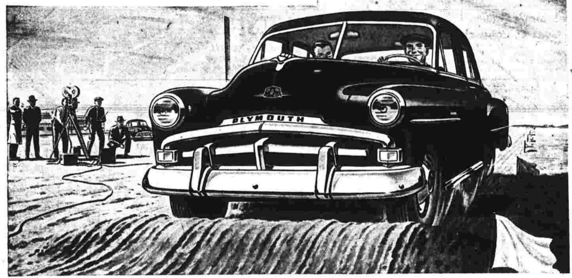
MOTION PICTURES made by our engineers show how little the new Plymouth goes up and down when passing over a bump, compared to cars that do not have the new "Safety-Flow Ride." New Oriflow shock absorbers, along with balanced weight distribution, synchronized springing, and other engineering features, hold the car closer to a level plane. They give Plymouth the riding qualities of a car weighing a thousand pounds more, in the opinion of Tom McCahill, automotive expert, writing in Mechanix Illustrated .
